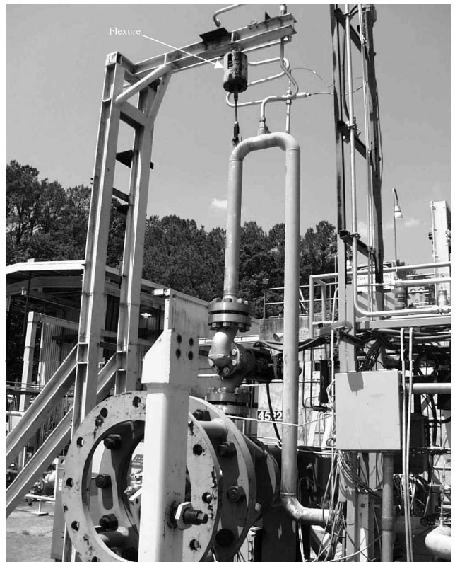
Fig. 5 LOX feed system.
